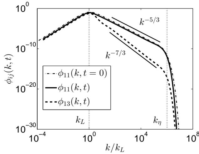
Figure 1. Second-order spectral tensors  $\phi_{13}(k, t)$  and  $\phi_{11}(k, t)$  for Saffman turbulence ( $\sigma = 2$ ), at  $t = 10\tau_0$  where  $Re_\lambda(10\tau_0) = 2.10^4$ . The shear rate is  $S = 1\tau_0^{-1}$  and the accumulated anisotropy is  $St = 10$ . The Kolmogorov wavenumber  $k_\eta$  and the integral wavenumber  $k_L$ , used for normalization, are indicated as well.
