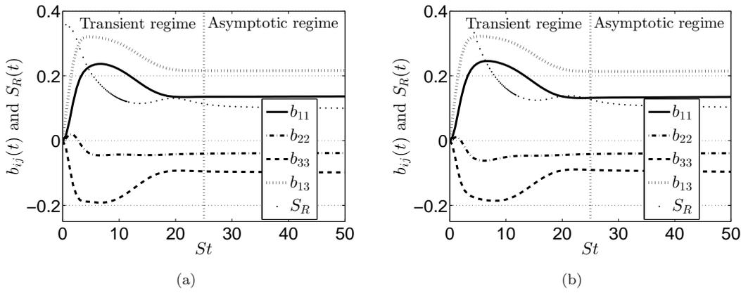
Figure 7. Anisotropy tensor  $b_{ij}(t)$  and shear rapidity  $S_R(t)$  with  $S = 1\tau_0^{-1}$ . (a)  $\sigma = 2$ . (b)  $\sigma = 4$ .
