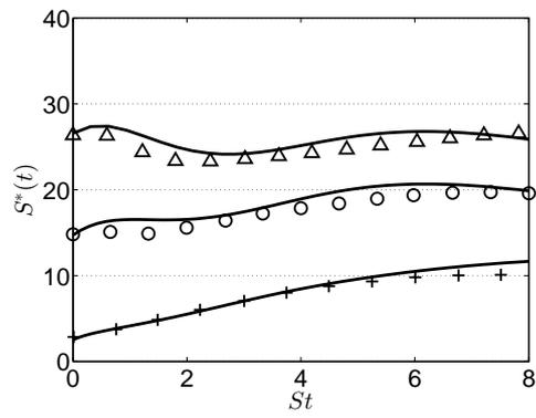
Figure B2. Evolution of the shear parameter  $S^*(t)$ . Comparison to the sustained shear flow DNS [41] with three different initial values  $S_0^*$ . Lines and symbols represent respectively the present EDQNM simulations and DNS: +,  $S_0^* = 3$ ; o,  $S_0^* = 15$ ; and  $\triangle$ ,  $S_0^* = 27$ .
