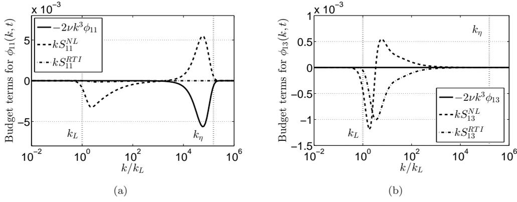
Figure 5. Budget terms of the evolution equation of the spectral tensor after the release of the shear:  $\partial_t \phi_{ij} = -2\nu k^2 \phi_{ij} + S_{ij}^{(NL)} + S_{ij}^{(RTI)}$ , at  $t = 10\tau_0$  for Saffman HSRT, where  $Re_\lambda = 7.10^3$ .  $S_{ij}^{(NL)}$  is the conservative part of the non-linear transfers, with zero integral over  $k$ , and  $S_{ij}^{(RTI)}$  is the remaining part, responsible for the RTI mechanism. (a) For  $\phi_{11}$ . (b) For  $\phi_{13}$ .
