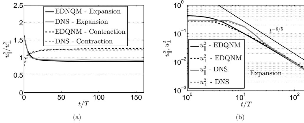
Figure B1. Grey lines correspond to the DNS and black ones to EDQNM. For the expansion,  $Re_{\lambda}(0) = 36$  and for the contraction  $Re_{\lambda}(0) = 25$ . (a) Ratio  $u_{\parallel}^2/u_{\perp}^2$  in axisymmetric expansion (plain line) and contraction (dashed line). (b)  $u_{\parallel}^2$  (plain line) and  $u_{\perp}^2$  (dashed line) decay in axisymmetric expansion only.
