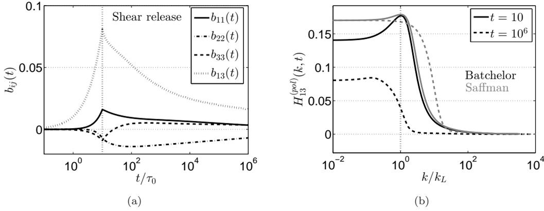
Figure 3. (a) Anisotropy tensor  $b_{ij}(t)$  for  $\sigma = 4$ . (b) Spectral anisotropy indicator  $H_{13}^{(pol)}(k,t)$  for Saffman ( $\sigma = 2$ , grey lines) and Batchelor ( $\sigma = 4$ , black lines) turbulence, at  $t = 10\tau_0$  and  $t = 10^6\tau_0$ . Both with  $S = 0.1\tau_0^{-1}$  and an injected anisotropy  $St = 1$ .
