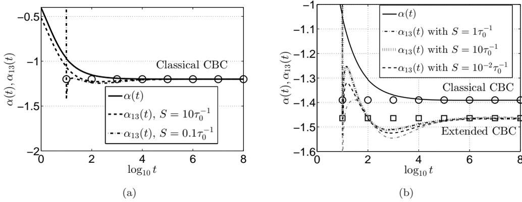
Figure 6. Decay exponents of  $K(t)$  and  $R_{13}(t)$  for various shear intensity  $S$ .  $\circ$ : Classical CBC exponents;  $\square$ : Extended CBC exponents. (a) Saffman HSRT:  $\alpha = \alpha_{13} = -6/5$ . (b) Batchelor HSRT:  $\alpha = -1.38$  is recovered.  $\alpha_{13} = -1.464$  with  $p_S = 0.279$ . The grey dash-dot curve  $- \cdot -$  corresponds to a distortion simulation with  $S = 1\tau_0^{-1}$ .
