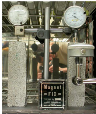
Figure 1. Experimental setup for shrinkage strain measurement
