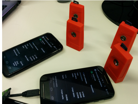
Fig. 4. ContextNet Mobile Hub with four SensorTags
