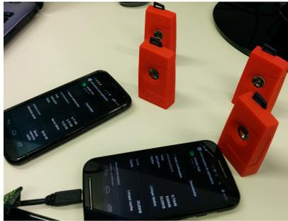
Fig. 4. ContextNet Mobile Hub with four SensorTags
