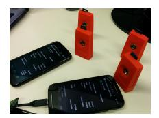
Fig. 4. ContextNet Mobile Hub with four SensorTags
