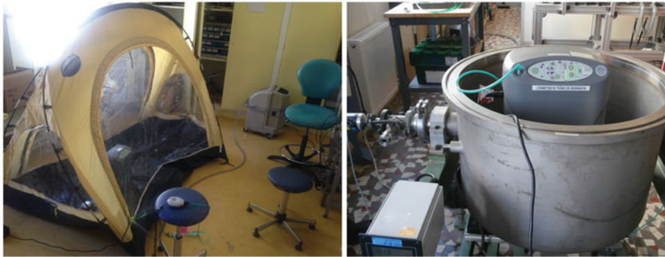
SUPPLEMENTARY FIG. S1. Setups used for measurements. Left: A portable oxygen concentrator in a hypoxic tent (hypoxic generator at the back of the room). Right: Portable oxygen concentrator in the altitude chamber.
