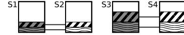
Fig. 3. Example of protection: master VNFs are running on servers S_2 and S_4 , while slave are running on S_1 and S_3 . Each link between VNF instances represents the connection between a master and its slave.
