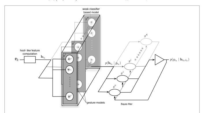
FIGURE 12 | Gesture Recognition Architecture: for each occurring hoof-like feature  $\mathbf{h}_{f_k}$ , the distribution of probabilities noted  $p(\mathbf{h}_{f_k} \mid g_{f_k})$ , is estimated comparing the features to models computed and selected through an Adaboost-based learning process. Then the probabilities of gestures, noted  $p(g_{f_k} \mid \mathbf{h}_{f_0:f_{k-1}})$ , are estimated recursively over time.
