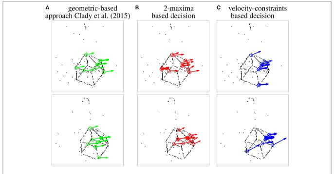
FIGURE 10 | Snapshots of the results obtained for the three compared detectors, projecting in a frame the visual events (black dots) and corner events (circles, associated to vectors representing the estimated speeds) over two short time periods (1 ms).
