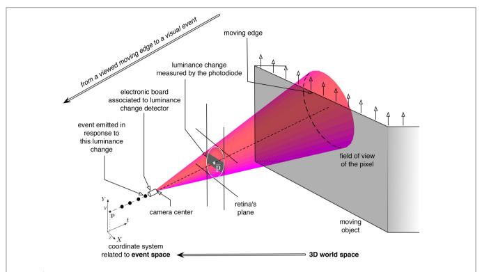
FIGURE 2 | Illustration of the luminance change measured by a neuromorphic pixel, modeled as a cone-pixel (Debaecker et al., 2010), viewing an moving edge. p are the coordinates of the center of the pixel, in the coordinate system related to the retina's plane. The emitted event in response to this luminance change is represented as a black dot in the coordinate system XYt related to the event space (in the lower-left part of the figure).
