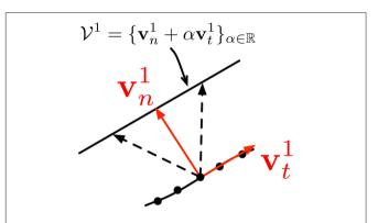
FIGURE 5 | The aperture problem allows estimating only the normal component  $\mathbf{v}_1^\eta$  of the velocity of events generated by an edge. The
