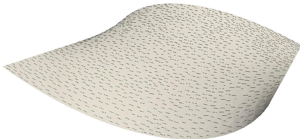
Figure 5: Initial fibre orientation (elliptic geometry shell)
