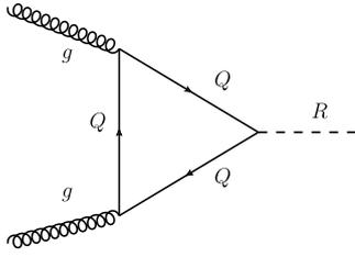
**Fig. 1.** Feynman diagram representing the loop-induced production of a scalar  $R$ -particle via gluon fusion when a heavy quark  $Q$  runs into the loop.
