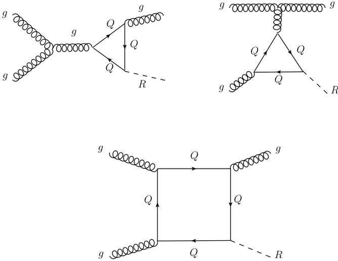
**Fig. 2.** Feynman diagrams representing the loop-induced production of a scalar particle  $R$  in association with a hard jet, via gluon fusion and when a heavy quark  $Q$  runs into the loop. The two diagrams in the first row are triangle ( $\Delta$ ) diagrams and the one in the second row is a box ( $\square$ ) diagram.
