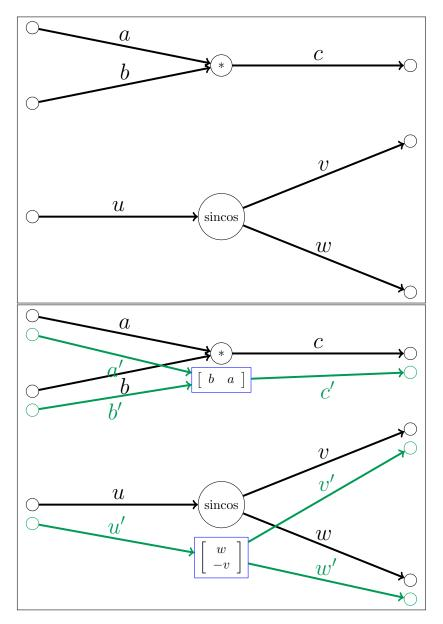
FIGURE 1. Forward AD augments all primitive arithmetic operations in the original flow graph (top) to also propagate derivatives forward through the computation (bottom).
