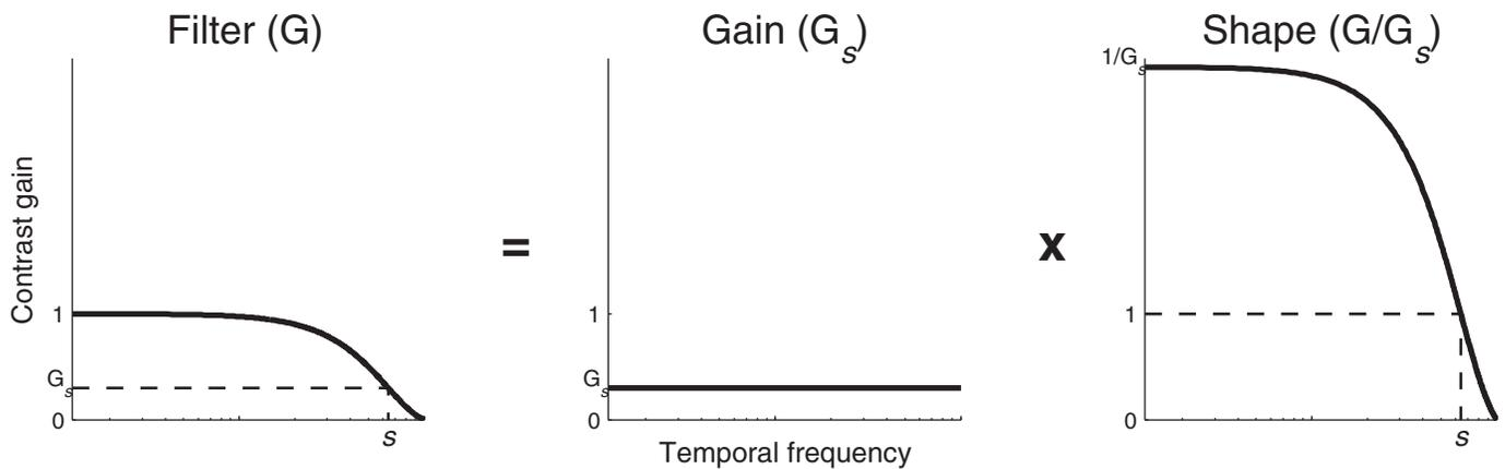
Figure 5. Given a signal temporal frequency ( $s$ ), a temporal filter ( $G$ , left graph) can be represented as a combination of two filters: a contrast gain at the signal frequency ( $G_s$ , center graph) and the normalized shape of the filter ( $G/G_s$ , right graph).
