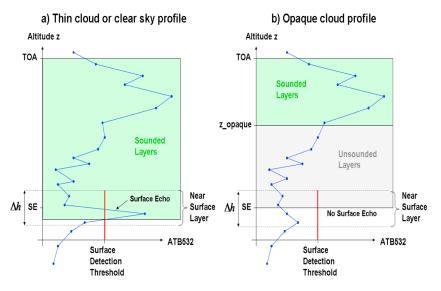
**Figure 1.** Surface echo detection scheme: ATB surface detection threshold (SDT) applied in a near-surface layer (NSL) extending from  $-\Delta h/2$  to  $+\Delta h/2$  with respect to the surface elevation (SE) for (a) a thin cloud or clear-sky profile case where the surface is detected and (b) an opaque cloud profile case where the surface is not detected.
