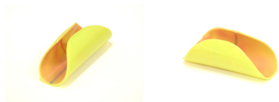
Fig. 9 Bifurcated shapes of the silicone shell corresponding to point C in Figure 3. The principal directions of curvature are marked on the shell in red and blue.
