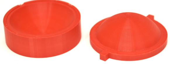
Fig. 11 Mold with radius of curvature 5.5 cm used to build the tristable shell in Figure 10.
