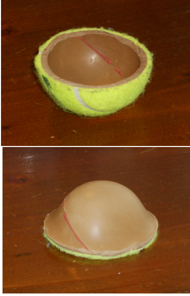
Fig. 7 Natural (a) and everted (b) configurations for half a tennis ball.
