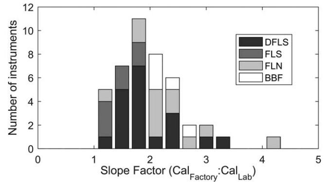
**Fig. 8.** Histogram of median slope factors for 55 WET Labs digital fluorometer sensors in the ECO series from 2001 through 2016. The slope factor for each sensor was computed over the lifetime of the sensor and comprises from 3 to 17 separate calibrations (factory and laboratory) depending upon the lifetime of the sensor.
