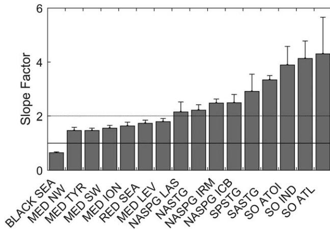
**Fig. 4.** Mean slope factors derived from ratio of factory calibrated Chl fluorescence to radiometrically-derived Chl (see text for details) obtained from profiling biogeochemical Argo floats described in Table 2. Error bars indicate 95% confidence limits on slope derived from regression of all observations within each region. Lines indicate slope factors of 1 (solid) and 2 (dotted).
