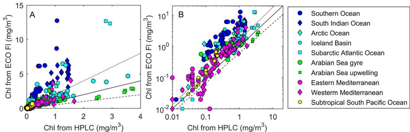
**Fig. 1.** Regression between factory-calibrated in vivo chlorophyll fluorescence observations from WET Labs ECO sensors and paired HPLC total Chl samples for the regions described in Table 1 on (A) linear and (B) log scales. Lines indicate slope factors of 0.5 (dash), 1 (solid), and 2 (dotted).
