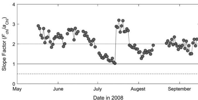
**Fig. 6.** Time series observations of the absorption-based slope factor derived from paired estimates of [Chl] from factory calibrated Chl fluorescence and ac9 absorption line height (Roesler and Barnard 2013) for 4 months in 2008. Data were collected from mooring D02 as part of the Gulf of Maine Ocean Observing System (GoMOOS) in Harpswell Sound, Casco Bay. Lines indicate slope factors of 0.5 (dash), 1 (solid), and 2 (dotted).
