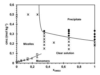
Figure 2: CMC and precipitation vs composition of the solvent. □: CMC by conductimetry. Δ: CMC from density measurements (molar volumes) •: solid samples. \*: clear, liquid samples. The solid lines are guides that indicate trends. Micelles are assigned on the basis of SANS data.
