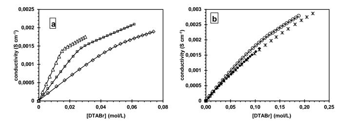
Figure 1: Conductivity data at 298 K (a)  $\Delta$ : water;  $\Box$ :  $x_{DMSO} = 0.06$  (20v%);  $\Diamond$ :  $x_{DMSO} = 0.14$  (40v%); (b) O:  $x_{DMSO} = 0.26$  (60v%);  $\bullet$ :  $x_{DMSO} = 0.35$  (70v%); \*:  $x_{DMSO} = 0.50$  (80v%). The straight lines correspond to the fit with equation (7) and the parameters listed in Table 2.
