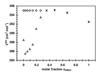
Figure 4: ( $\Delta$ ) Apparent molar volumes in the monomeric form at the CMC  $V_{CMC}$  and ( $\Diamond$ ) in the micellar phase  $V_{mic}$  for conditions in which they can be determined separately. (\*) indicate an equal value of V for monomeric or micellar species throughout the molality range of DTABr. T = 298.0 K.
