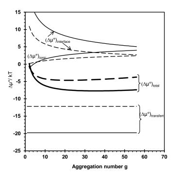
Figure 10: Free enthalpy contributions calculated according to Nagarajan's model. Solid lines:  $x_{DMSO} = 0$ ;  $C_{tot} = 1.12 \times 10^{-2}$  mol  $L^{-1}$  and  $X_1 = 0.000203$ . Dashed lines:  $x_{DMSO} = 0.26$ ;  $C_{tot} = 1.32 \times 10^{-1}$  mol  $L^{-1}$  and  $X_1 = 0.0038$
