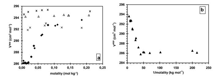
Figure 3: Apparent molar volumes  $V^{app}$  vs. molality of DTABr in water-DMSO mixtures. T =298.0 K. (a)  $\bullet$ :  $x_{DMSO} = 0.06$  (20v%); \*:  $x_{DMSO} = 0.50$  (80v%);  $\Delta$ :  $x_{DMSO} = 0.67$  (90v%); \*:  $x_{DMSO} = 1$ . (b) Apparent molar volume of solutions  $V^{app}$  vs. reciprocal of molality in water-DMSO mixtures ( $x_{DMSO} = 0.06$  (20v%).
