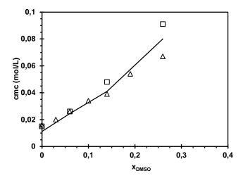
Figure 11: Comparison of calculated (solid line) CMC values to experimental CMC values determined from density measurements ( $\Delta$ ) and from conductivity measurements ( $\Box$ ).
