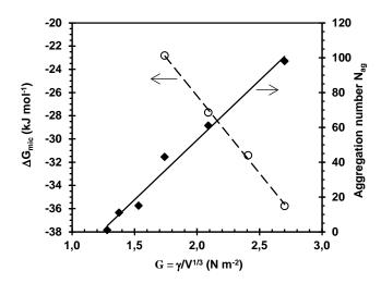
Figure 7: Plots of the molar free enthalpy of micellization  $\Delta G_{mic}$  (O) and the aggregation number  $N_{ag}$  ( $\blacklozenge$ ) vs the Gordon parameter G of solvents having various DMSO contents (obtained from Figure 6). The lines are visual guides.
