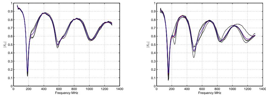
Figure .10: The measurements of the reflection coefficient  $S_{11}$  (black), predicted values with LS-SVM (blue) and with neural network (red) for MC = 30% (left) and MC = 48% (right) with the 54 cm length antenna for softwood.
