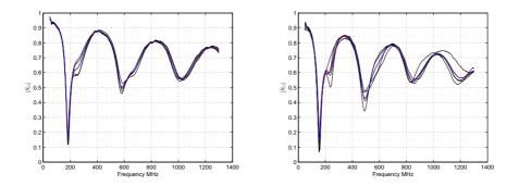
Figure .10: The measurements of the reflection coefficient  $S_{11}$  (black), predicted values with LS-SVM (blue) and with neural network (red) for MC = 30% (left) and MC = 48% (right) with the 54 cm length antenna for softwood.
