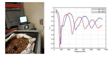
Figure 1: The laboratory-scale measurement system (left). Modulus of  $S_{11}$  of the 54 cm length antenna for two MC values (right).
