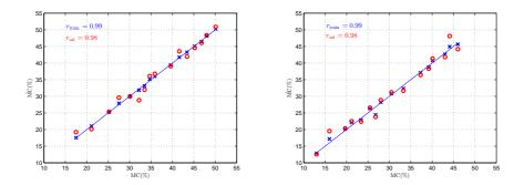
Figure 8: The MC predicted values when Gram-Schmidt + LS-SVM with linear kernel is applied to softwood (left) and hardwood (right) with the half-wave dipole antenna 54 cm.
