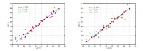
Figure 9: The MC predicted values when Gram-Schmidt + LS-SVM with linear kernel is applied to mixture of wood with both antenna lengths 45 cm (left) and 54 cm (right). The training errors are in blue, validation errors are in red and test errors are in green.
