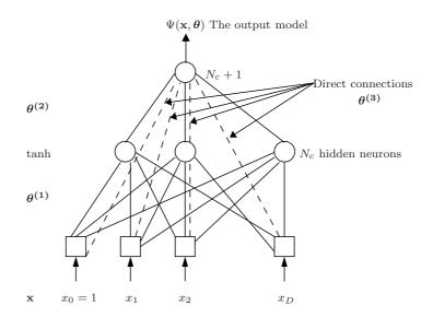
Figure 4: A feedforward neural network with direct connections.
