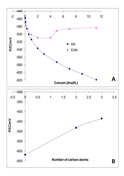
**Fig. 5.** (A) Variation of PZC as a function of the EAN concentration with respect to that of AN, (B) Relationship between PZC and number of the carbon atoms present within the ammonium cation (AN, EAN and PAN).
