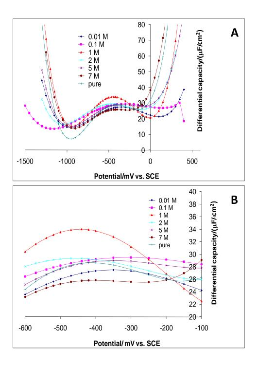
**Fig. 7.** (A) Differential capacitance as a function of the potential for the various EAN concentrations, (B) Zoom of (A) around PZC.
