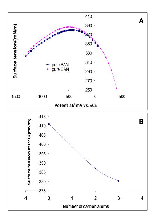
**Fig. 4.** (A) Comparison between the electrocapillarity curves of pure EAN with respect to pure PAN, (B) Relationship between surface the tension at PZC and number of the carbon atoms present within the ammonium cation (AN, EAN and PAN).
