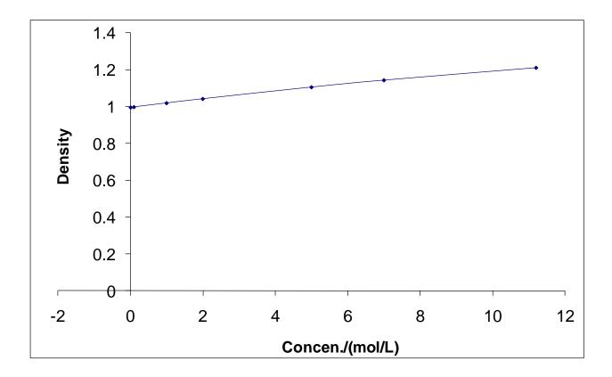
Fig. 2. Variation of density of EAN-water mixtures as a function of the EAN concentration.
