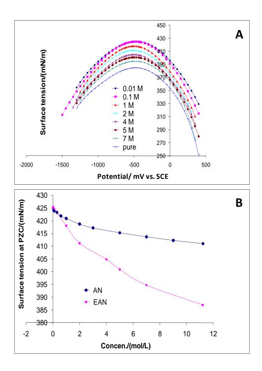
**Fig. 3.** (A) Electrocapillarity curves of EAN-water mixtures at various EAN concentrations, (B) Comparison between the curves of surface tension at PZC as a function of the concentration of EAN and AN.
