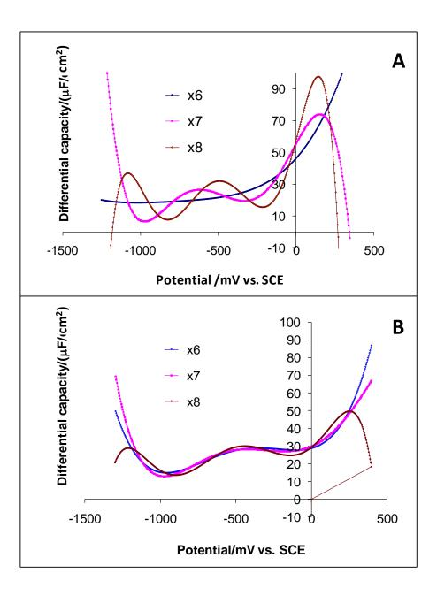
**Fig. 9.** Variation of the differential capacitance with the polynomial regression fitting order of 6, 7 and 8 for EAN at 7 M (A) and 5 M (B).
