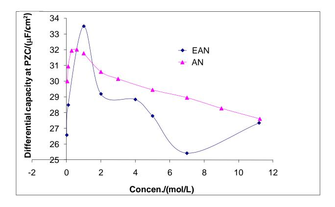
**Fig. 8.** Variation of the differential capacity at the PZC as a function of the concentration of EAN and AN.
