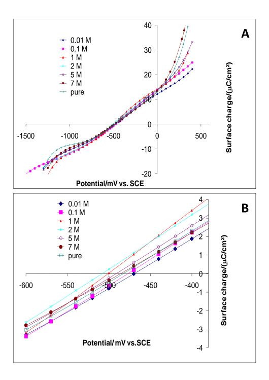
**Fig. 6.** (A) Surface charge on the mercury electrode as a function of the potential at various EAN concentrations, (B) Zoom of (A) around the PZC.
