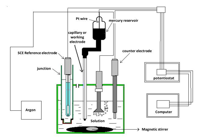
Fig. 1. Schematic representation of the dropping mercury electrode (DME) system used in this study.
