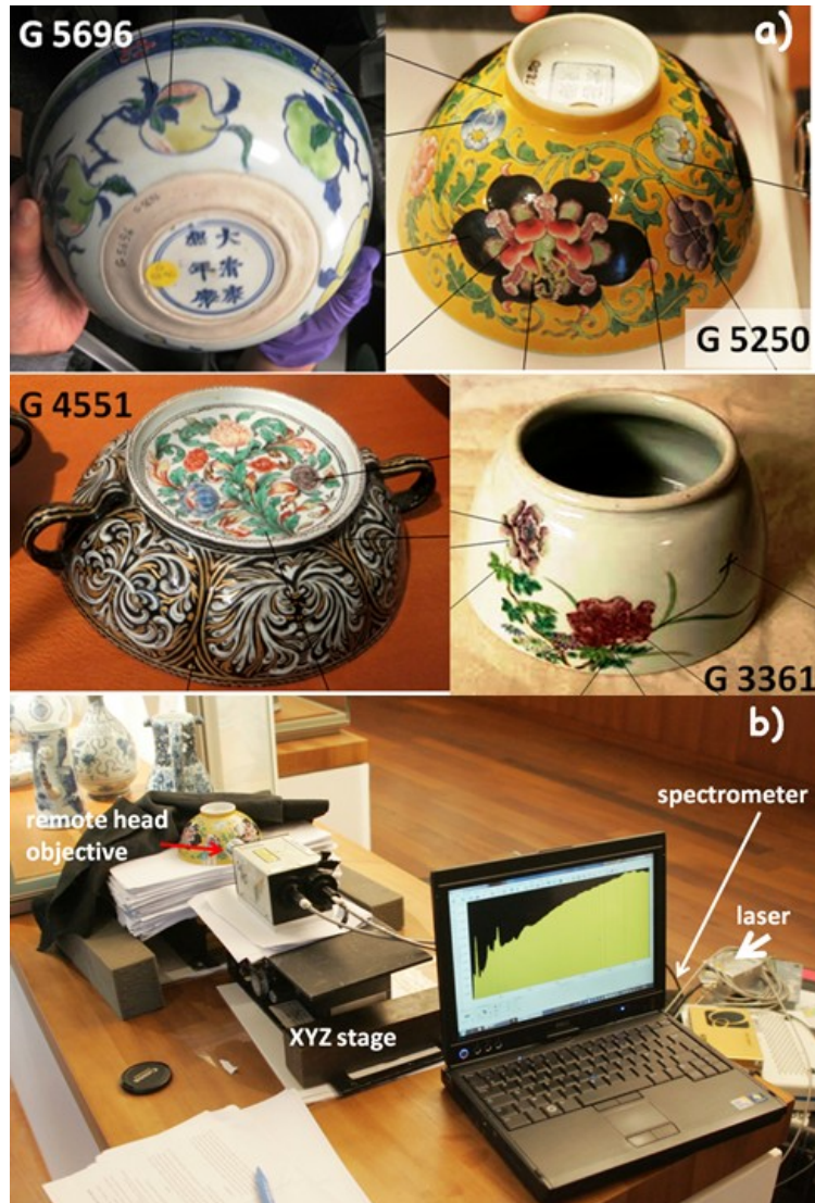
Fig. 1: a) Representative Qing Dynasty porcelains made respectively with ' Couleurs transparentes ' (G 5696) and opaque/ huafalang (G 5250, G 4551 and G 3361) enamels.(see Table 1 and Supplementary Materials for details; b) mobile Raman set-up.
