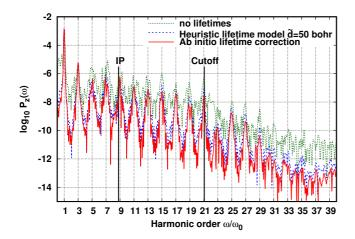
FIG. 5: HHG spectra of the H atom with laser intensity  $I=10^{14}~{\rm W/cm^2}$  calculated with the 6-aug-cc-pVTZ+8K+pd( $\alpha_{\rm min,s}$ ) basis set using either no lifetimes, the lifetimes from the heuristic lifetime model [21] using  $\tilde{d}=50$  bohr or the lifetimes from our *ab initio* lifetime correction. The vertical lines correspond to the value of the IP and the three-step model energy cutoff [48, 49].
