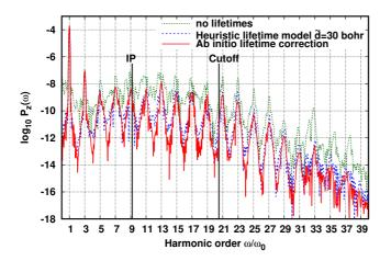
FIG. 7: HHG spectra of the He atom with laser intensity  $I=5\times 10^{14}~{\rm W/cm^2}$  calculated with the 6-aug-cc-pVTZ+7K+pd( $\alpha_{\rm min,s}$ ) basis set using either no lifetimes, the lifetimes from the heuristic lifetime model [21] using  $\tilde{d}=30$  bohr or the lifetimes from our *ab initio* lifetime correction. The vertical lines correspond to the value of the IP and the three-step model energy cutoff [48, 49].
