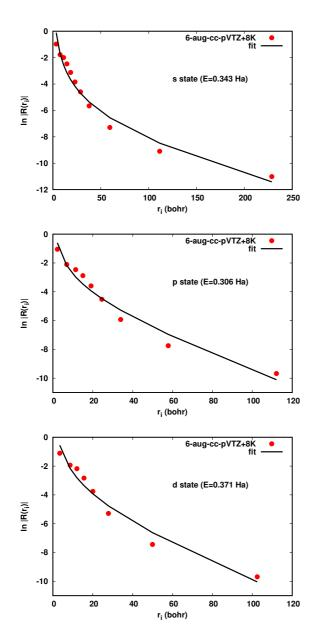
FIG. 2: Fit to the logarithmic formula of Eq. (21) of the envelope of the s, p, and d radial wave functions R(r) of the H atom with positive energies of 0.343 Ha, 0.306 Ha, and 0.371 Ha, respectively, calculated with the 6-aug-cc-pVTZ+8K basis set. The points defining the envelope are defined as the maxima  $r_i$  of |R(r)|. The coefficients of determination  $R^2$  of the fit are 0.97, 0.96 and 0.96, respectively.
