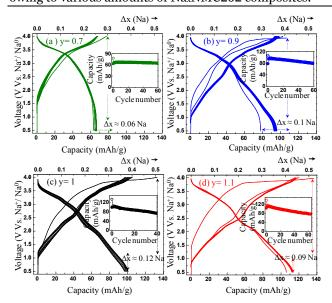
Figure 9: Voltage profile with the capacity retention plot as inset of the full cells assembled with P2 Na<sub>x</sub>NMC262 phases (a) y=0.7, (b) y=0.9, (c) y=1 and (d) y=1.1; the reversible capacity of the full cells increased with increasing y and hence increasing amount of Na<sub>2</sub>CO<sub>3</sub> sacrificial salt in the composite.
