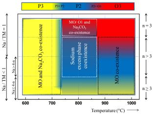
Figure 6: Synthesis phase diagram of  $Na_xMO_2$  as a function of temperature, Na/TM ratio and the total oxidation state on the transition metal layer (n). In the formula, M is one or more transition metal ions in which the ion such as  $Mn^{4+}$  with smaller ionic radius and high charge (+4) is in high proportion of 0.6 or more.
