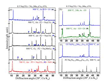
Figure 5: Powder X-ray diffraction patterns of the (a)  $Na_xNMC262$ , y=1.1 prepared at different temperature and in different environment, (b)  $Na_xNMC550$ , y=1.1 at 800 °C in air and Argon atmosphere, (c)  $Na_xNi_{0.16}Mn_{0.33}Fe_{0.5}O_2$ , y=1.1 and  $Na_xNi_{0.22}Mn_{0.66}Fe_{0.11}O_2$ , y=1.1 synthesized in air at 800 °C.
