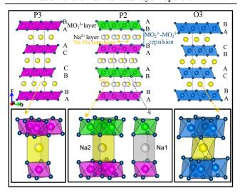
Figure 1: Structure (top) and the sodium coordination (bottom) of P3, P2 and O3 phases. The figure is plotted using the structural data from ref. 19, 26
