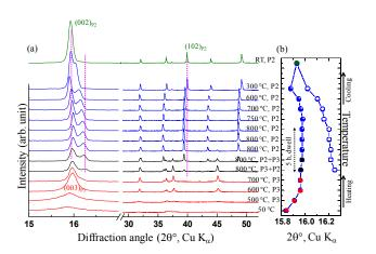
Figure 4: (a) High temperature XRD pattern of the  $Na_xNMC262$  precursor with y=1. The pink lines are guide to eye to follow the variations in  $(002)_{P2}$  and  $(102)_{P2}$  peak positions (b) Variation in  $(003)_{P3}/(002)_{P2}$  peak position with temperature.
