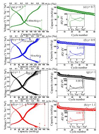
Figure 7: Galvanostatic charge- discharge profiles of P2  $Na_xNMC262$  prepared with Na/TM ratio 'y' of (a) 0.7, (b) 0.9, (c) 1 and (d) 1.1; the difference in capacity between the first cycle charge and discharge are denoted in the cycling curves and the capacity due to the plateau at 4V are also marked in the voltage profile. (e- h) the capacity retention plots and the derivative curve as inset for (e) y=0.7, (f) y=0.9, (g) y=1 and (h) y=1.1.
