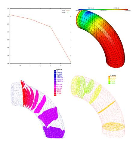
Figure 5: Top left: Optimization criteria versus iteration number. Top right: the coefficient b(x) after 3 iterations. Bottom Left: effect of the change of b on the dilatation of the vessel and some iso surfaces of constant pressure. Bottom right: a snap shot of the adjoint pressure and some iso surfaces.
