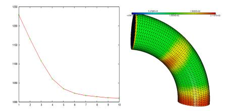
Figure 6: Left: Optimization criteria  $\int_{\Sigma \times (0,T)} p^4$  versus iteration number. Right: the coefficient b(x) after 4 iterations. Right: effect of the change of b on the dilatation of the vessel.
