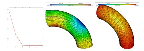
Figure 7: Left: Optimization criteria  $\int_{\Sigma \times (0,T)} (p-p_d)^2$  versus iteration number. Right: the coefficient b(x) after 5 iterations. middle: The target b.
