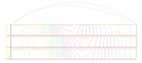
Figure 3: Target  $b_d$  (top curve) and computed b after 50 iterations. Initial Pressure map after one iteration (top), final pressure after 50 gradient iterations (middle) and target pressure  $p_d$  (bottom). The color scales are linear from -986 to 896 except for  $p_0$  which has a range from -680 to 782
