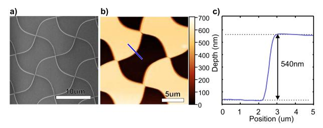
**Figure 3.** Fabrication and characterization of the  $0.84 \times \pi$  grating. (a) Electron microscopy image of the resulted grating showing a good border definition of the different etching zones. (b) Scanning AFM image of the heights of the gratings as a convolution of the physical size of the tip and the real structure of the grating. The cross section along the blue line is presented in (c).
