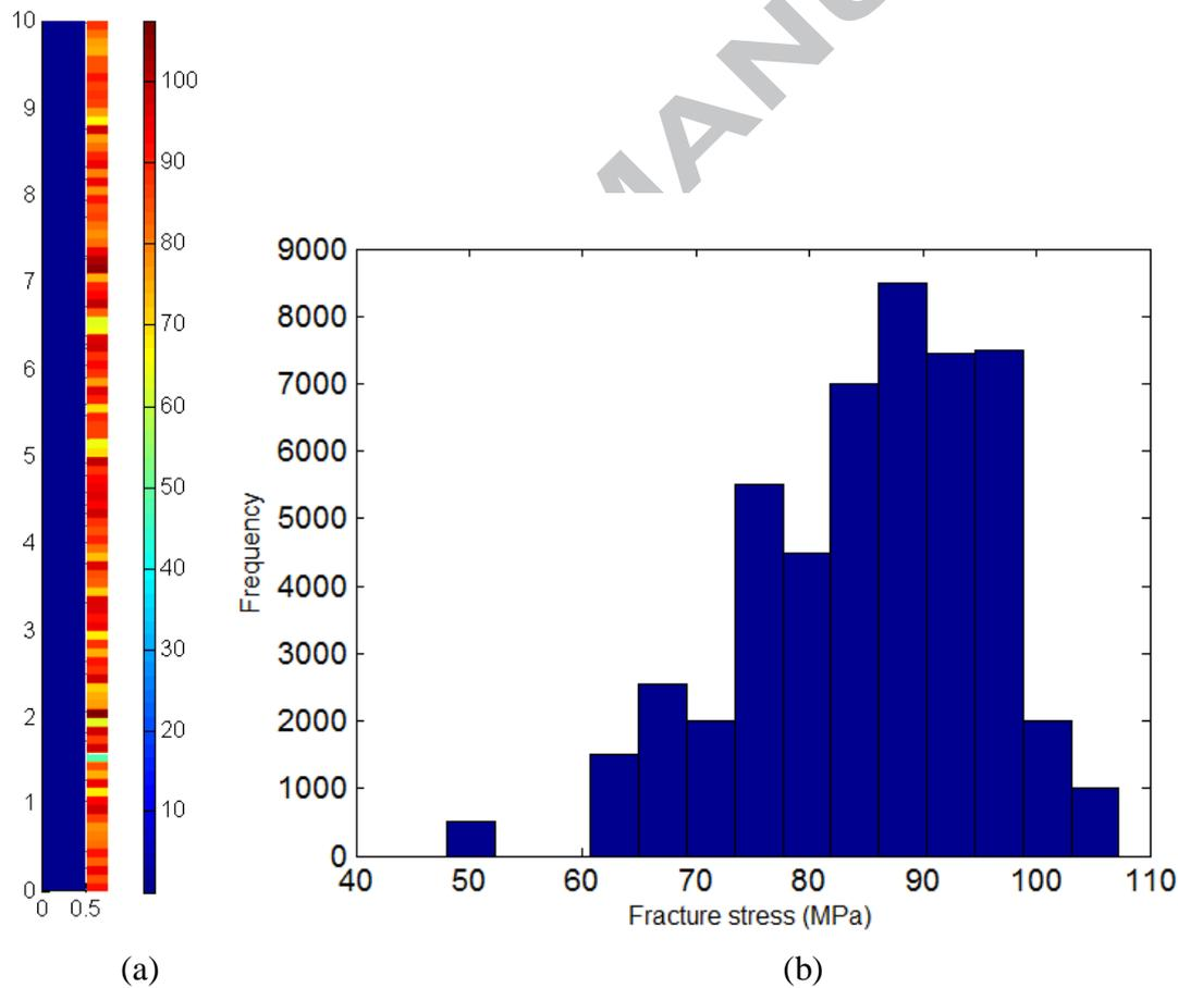
Figure 12: (a) Strength distribution in the inner ply according to the Weibull model (b) Histogram of strength
