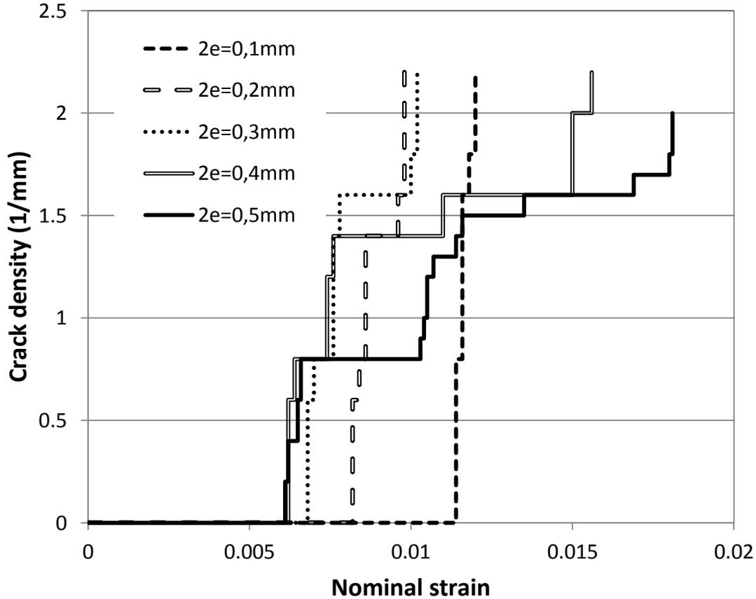
Figure 11: Crack density as function of Nominal strain for different thickness of the inner ply
