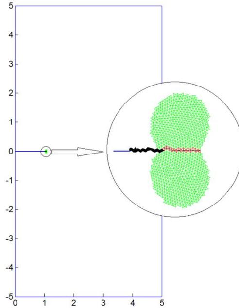
Figure 5: Growth simulation of a central crack. The black band represents the removed elements after the first step of the crack growth.
