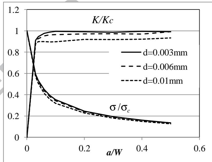
Figure 6: Normalized stress intensity factor  $K_I/K_{Ic}$  and normalized remote stresses  $\sigma^\infty/\sigma_c$  as a function of the normalized semi-crack length  $a/W$  for mode-I loaded cracks at fracture.
