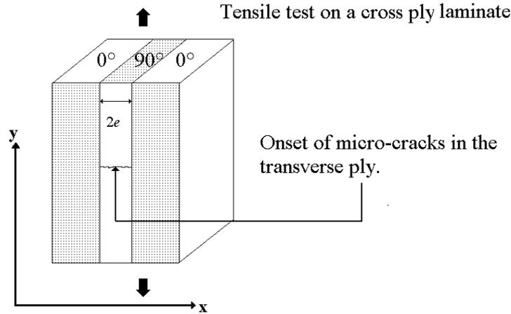
Figure 8: Scheme of the tensile tests on a cross-ply glass fiber-reinforced composite Include the
