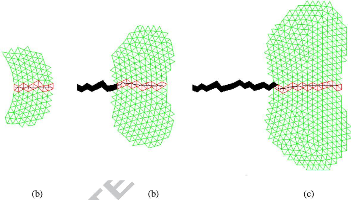
Figure 3: Numerical simulation of the crack initiation and growth (a): crack onset from the hole boundary (b)-(c): crack growth under unchanged remote displacement load
