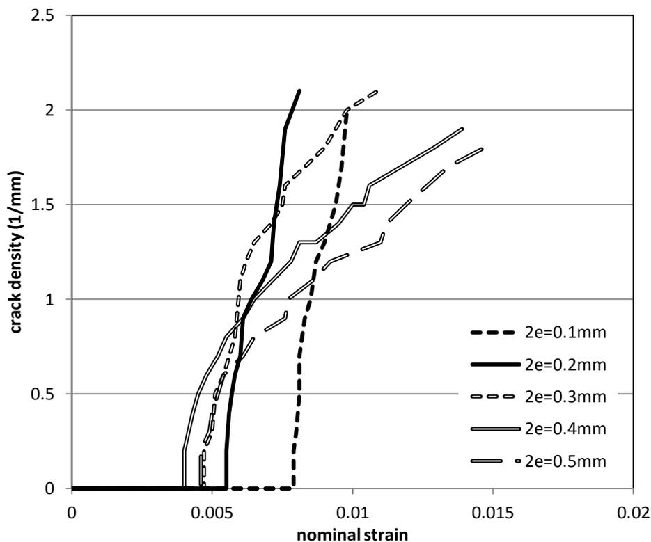
Figure 13 Crack density as function of Nominal strain for different thickness of the inner ply according to the Weibull model
