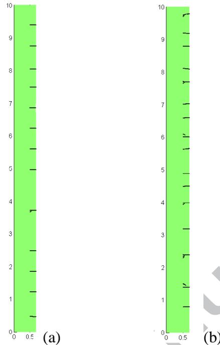
Figure 14: Crack patterns in the inner ply obtained by using the deterministic (a) and probabilistic (b) approaches respectively at nominal strain  $\varepsilon = 0.0115$
