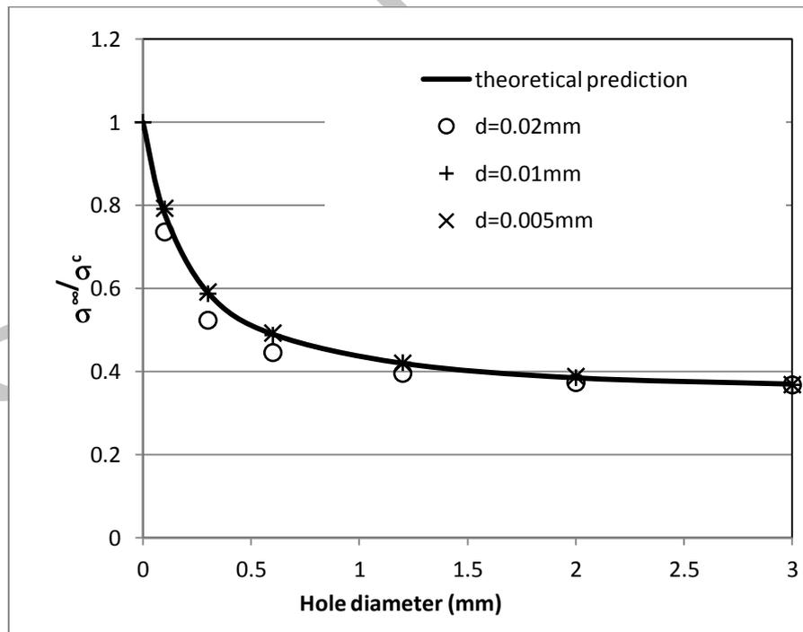
Figure 2: Critical remote stress at fracture of the drilled specimens as function of the hole size. Comparison between the theoretical and numerical predictions
