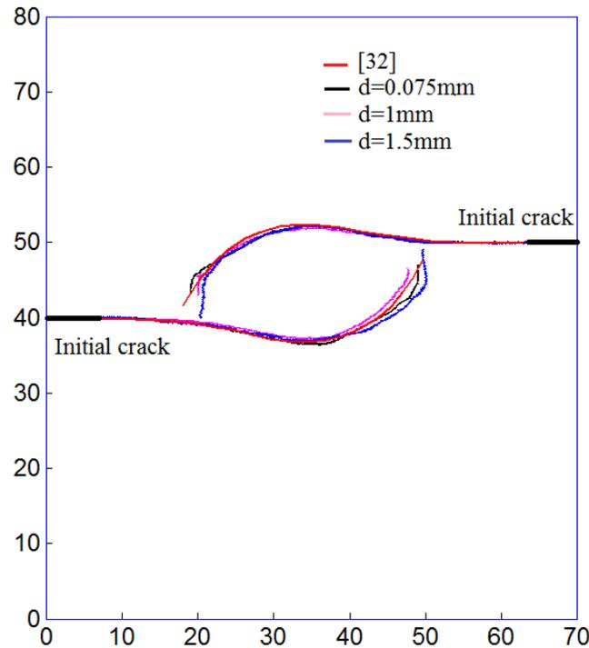
Figure 7: Crack paths predicted by using different meshes in a plate with double cracks
