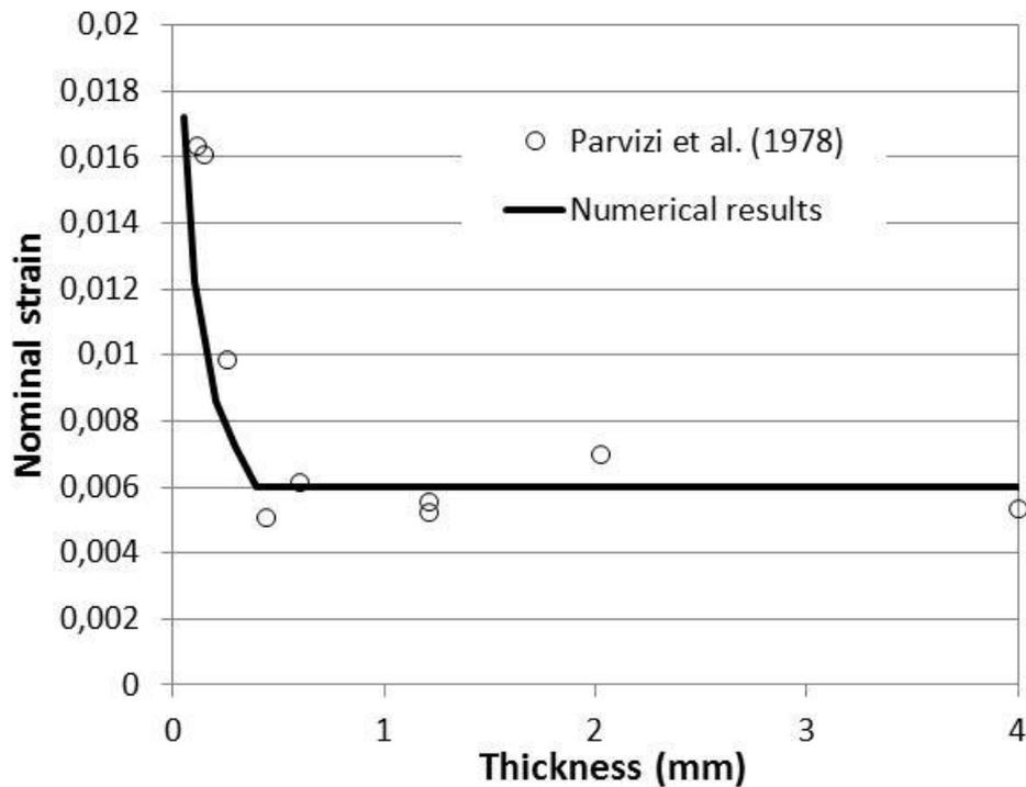
Figure 10: Nominal strain at the occurrence of the first transverse crack versus the thickness of the inner ply
