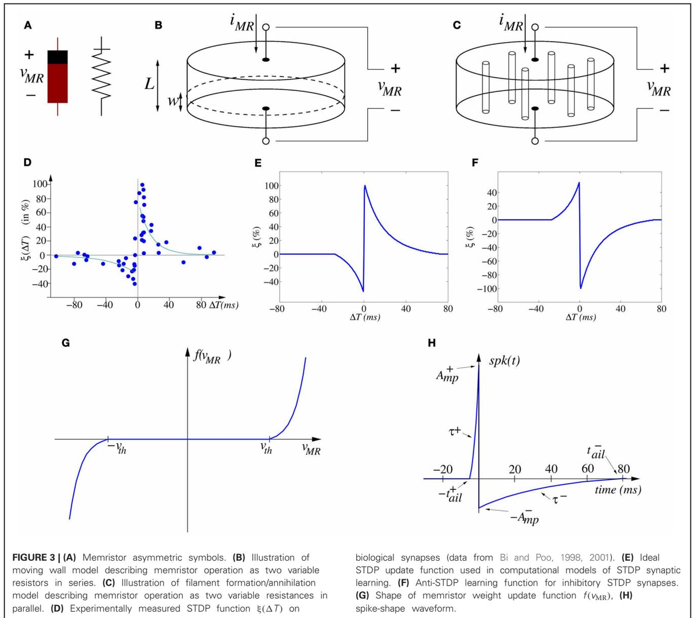
and down with the amount of charge that has flown through the memristor (in the case of being current/charge driven) or the accumulated flux (in case of being voltage/flux driven). The memristor would behave as two variable resistors in series. The total effective resistance of the memristor would be described by
