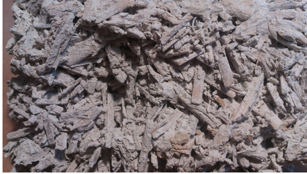
(a) Close up of a hemp and lime concrete sample
