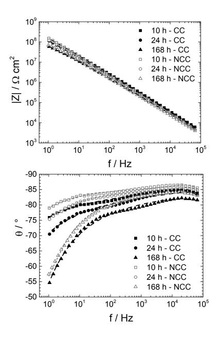
Fig. 3: Impedance responses in Bode format for the AA2024 coated samples (CC and NCC) after 10 h, 24 h and 168 h of immersion in 0.5 M NaCl solution. The solid lines are the best fitted curves according to Eq. (7).
