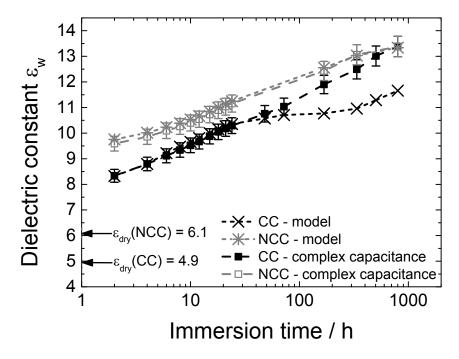
Fig. 6: Comparison of the wet dielectric constant ( $\varepsilon_w$ ) obtained from the impedance data analysis (in the frequency range 65 kHz to 1 Hz) and from the complex-capacitance plots at 65 kHz.
