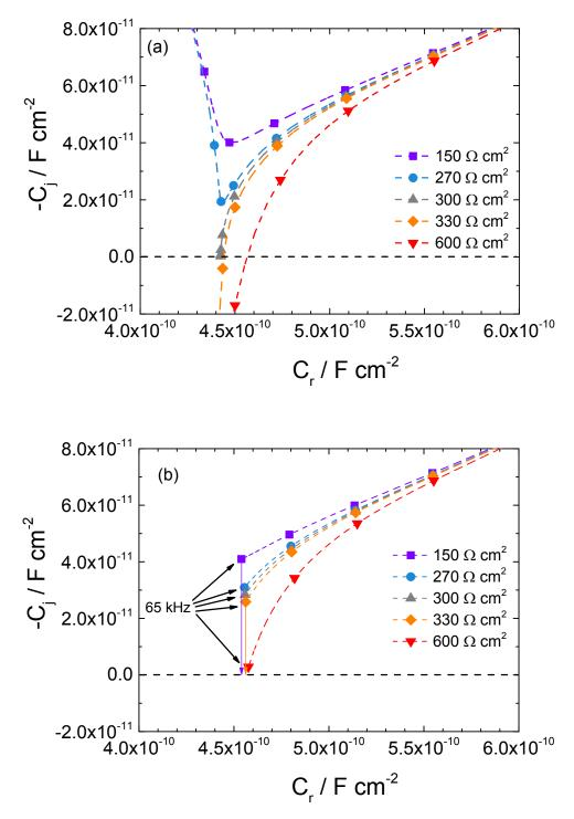
Fig. 2: Influence of the  $R_e$  value used for the conversion of the calculated impedance shown in Fig. 1 to capacitance. Complex-capacitance plots are shown for the  $R_e$  values indicated on the figure. (a) high frequency region and (b) same curves truncated at 65 kHz (measured frequency limit in this work)
