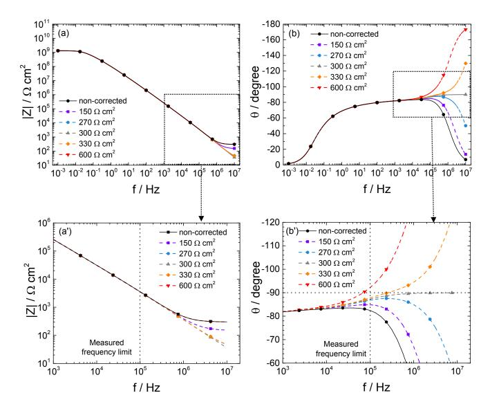
Fig. 1: Synthetic impedance calculated for a Young impedance, Eq. (6), in series with an electrolyte resistance, with:  $\delta = 20 \ \mu m$ ,  $\rho_0 = 10^{13} \ \Omega \ cm$ ,  $\lambda = 1.3 \ 10^{-4} \ cm$ ,  $\varepsilon_w = 10$ ,  $R_e = 300 \ \Omega \ cm^2$ . The uncorrected curves and curves corrected with different  $R_e$  values indicated on the figure are shown. Parts (a') and (b') are expanded views of parts (a) and (b), relevant to the high frequency region.
