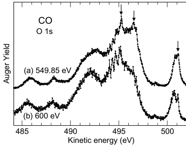
**Figure 1.** O 1s Auger spectrum of CO in the kinetic-energy region between 484 and 502 eV measured at a photon energy of (a) 549.85 eV and (b) 600 eV. Three spectral features, which are only visible in the spectrum measured at 549.85 eV, are marked by vertical arrows.
