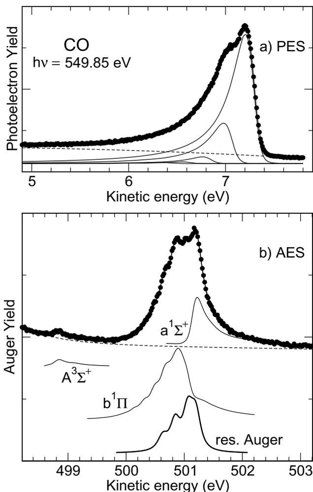
**Figure 4.** (a) Photoelectron and (b) Auger spectra recorded at a photon energy of 549.85 eV. The bold solid subspectrum in the AES represents the contributions of the resonant Auger decays of the doubly excited state. For more details, see figure 3.
