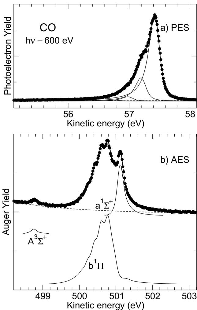
**Figure 3.** (a) Photoelectron and (b) Auger spectra recorded at a photon energy of 600 eV. In both spectra, the solid lines through the data points represent the fit results and the dashed lines indicate the background. In the PES the subspectra represent the different vibrational substates of the core-ionized state, while in the AES the subspectra indicate the vibrational progressions of the Auger decays to the final states  $a^1\Sigma^+$ ,  $b^1\Pi$  and  $A^3\Sigma^+$ .
