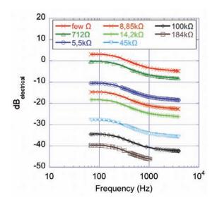
Figure 6: Variations of  $V_{\rm bag}$  according to the frequency with different resistances: from top to bottom, resistance increases from few  $\Omega$  to  $184 \,\mathrm{k}\Omega$ .
