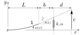
Figure 10: Mechanical model of the key, with beam 1 of length L, bar 2 of length b+d.
