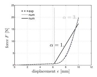
Figure 11: Force-displacement curves: experimental (black dash line), numerical fitting with E = 200 GPa,  $\alpha = 3., k = 40.0$  N.mm<sup>-1</sup> (gray solid line), and reference curve  $\alpha = 1$ . (black solid line).
