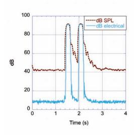
Figure 7: Measurements of the time signals of the electric amplitude after the powder bag,  $dB_{elec}$  (solid blue line), and the absolute  $dB_{SPL}$  from the microphone (dash brown line), during a double staccato (note  $C_3$ ), from no sound to fortissimo, color online.
