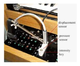
Figure 4: Intensity key instrumented with sensors.
