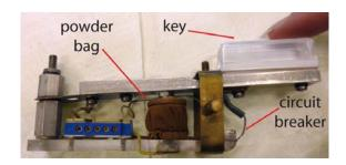
Figure 3: The intensity key removed from its drawer.
