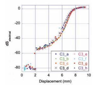
Figure 8: Variations of dB<sub>elec</sub> according to key's displacement, for a fixed note  $(C_3)$ .
