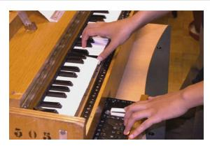
Figure 1: Playing the Ondes Martenot using the keyboard: right hand controls the pitch of the note while left hand adjusts the volume by pressing the intensity key.
