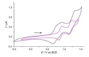
**Figure 7.** Cyclic voltammograms of compounds **16** (pink) and **20** (purple) on a Pt electrode in  $CH_2Cl_2+0.1$  M [ $nBu_4N$ ][BF<sub>4</sub>] at a scan rate of 200 mV s<sup>-1</sup> (toward anodic potentials).
