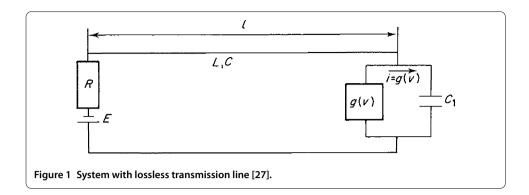
long electrical line (cable) of length l, one end of which is switched on a power source E with resistance  $R_E$ , while the other end is switched on an oscillating circuit formed by a condenser  $C_1$  and a nonlinear element, the volt-ampere characteristic of which is i = g(v) (Figure 1).
