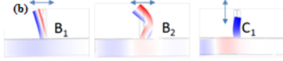
Figure 2. (a) Resonance frequencies of a single pillar (black and red lines) or a line of pillars (green and blue lines). The dimensions are (in \mu\text{m} ) h=245 , d=50 , t=145 , \theta=0^\circ . (b) Cartography of the displacement fields at resonance. The red (blue) color corresponds to a positive (negative) displacement with a zero represented with the white color. The deformations have been magnified for better observation.
