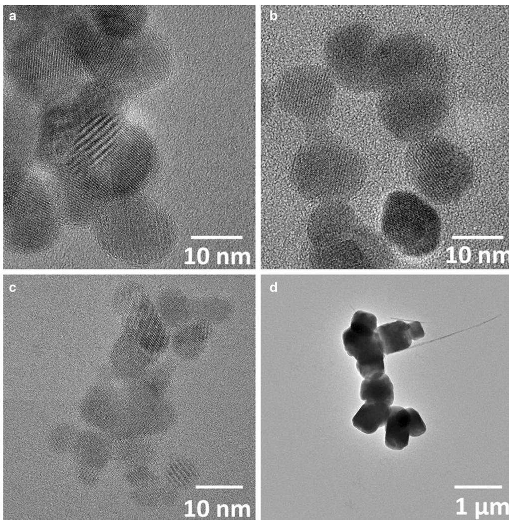
**Fig. 1** Transmission electron micrographs (bright field) of the initial magnetite particles: **a** biogenic magnetite, **b** 13 nm magnetite, **c** 7 nm magnetite, and **d** 500 nm magnetite
