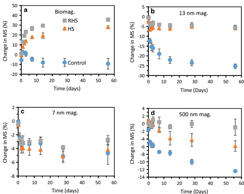
**Fig. 5** Magnetic susceptibility over time for 1 g/L of **a** biogenic magnetite, **b** 13 nm magnetite, **c** 7 nm magnetite, and **d** 500 nm magnetite in the absence of HS (blue filled circles), presence of native HS (orange filled triangles) and reduced HS (grey filled squares). Standard deviations of all experiments were calculated from three independent parallels
