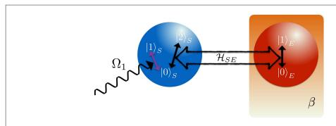
**Figure 1.** Scheme of the physical system considered. A three-level V-system is coupled to a two level environment which is at thermal equilibrium and the  $|0\rangle_S - |1\rangle_S$  transition is externally pumped.
