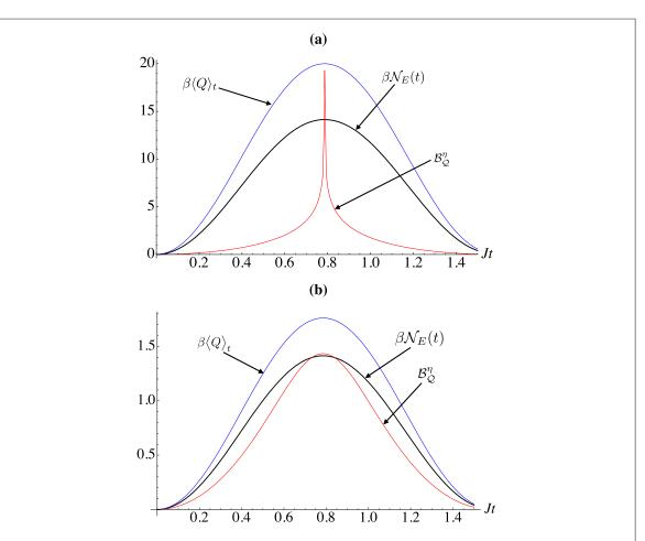
**Figure 3.** Mean dissipated heat  $\beta \langle Q \rangle_t$  (top-most blue curve), rescaled non-unitality  $\beta \mathcal{N}_E(t)$  (middle, black curve) and the lower bound  $\mathcal{B}_Q^{\eta}$  for  $\eta = \beta$  (bottom-most red curve). In both panels, we set B = J = 1,  $\Omega_1 = 0.1$  and take  $\beta = 10$  ( $\beta = 1$ ) in panel (a) ((b)).
