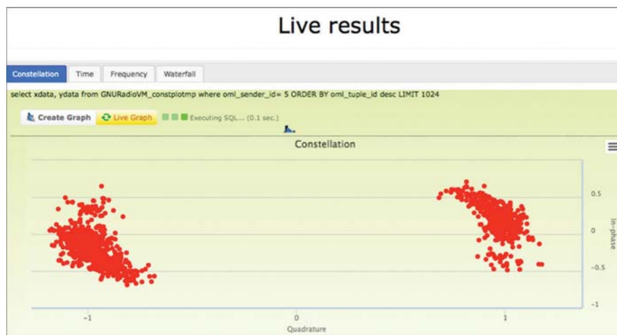
Figure 17.22 Real-time constellation measurements.
