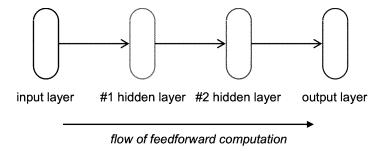
Fig. 5.13 Example of a feedforward neural network (abstract)
