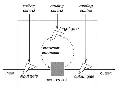
Fig. 5.34 LSTM architecture (conceptual)
