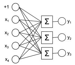
Fig. 5.5 Architectural model of multivariate linear regression
