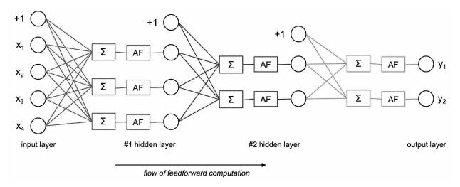
Fig. 5.11 Example of a feedforward neural network (detailed)
