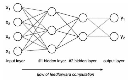
Fig. 5.12 Example of feedforward neural network (simplified)
