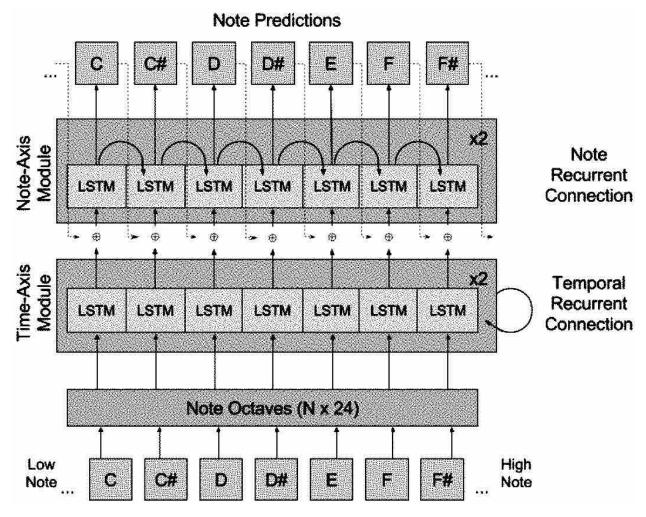
Fig. 6.29 Bi-Axial LSTM architecture. Reproduced from [127] with permission of the authors
