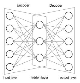
Fig. 5.22 Autoencoder architecture
