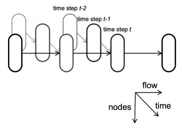
Fig. 5.29 Recurrent neural network (unfolded)
