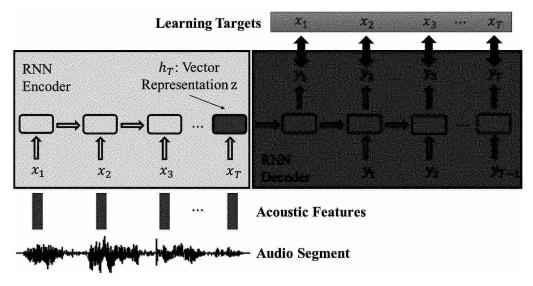
Fig. 5.43 RNN Encoder-Decoder audio Word2Vec architecture. Reproduced from [26] with permission of the authors
