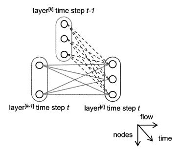
Fig. 5.30 Standard connexions versus recurrent connexions (unfolded)
