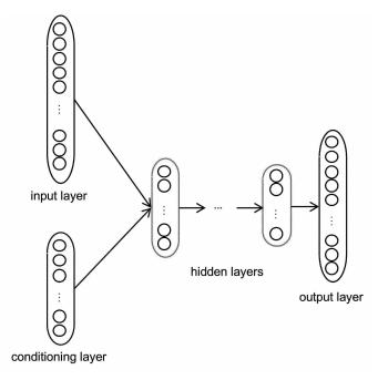
Fig. 5.38 Conditioning architecture
