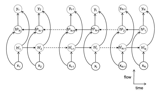
Fig. 5.41 Bidirectional RNN architecture
