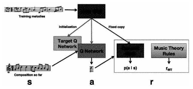
Fig. 6.60 RL-Tuner architecture. Reproduced from [93] with permission of the authors
