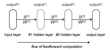
Fig. 5.20 Example of a feedforward neural network (abstract) pipelined computation
