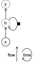
Fig. 5.31 Recurrent neural network (folded)
