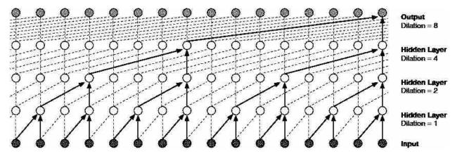
Fig. 6.39 WaveNet architecture. Reproduced from [194] with permission of the authors
