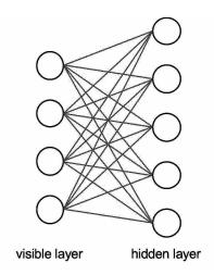
Fig. 5.27 Restricted Boltzmann machine (RBM) architecture
