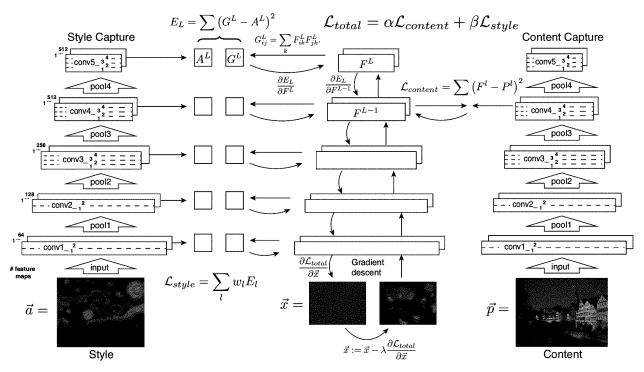
Fig. 6.53 Style transfer full architecture/process. Extension of a figure reproduced from [56] with permission of the authors
