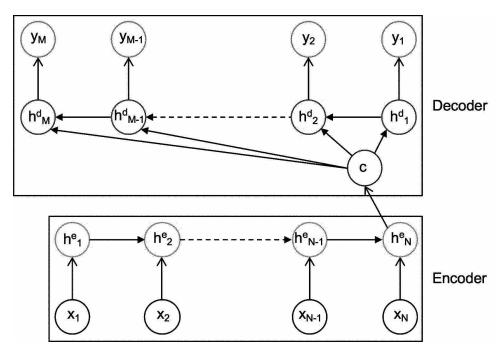
Fig. 5.42 RNN Encoder-Decoder architecture. Inspired from [20]
