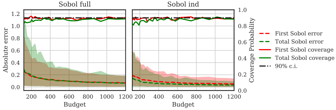
Figure 6: Variation of the absolute error and the POC with the computational budget for the RT method.
