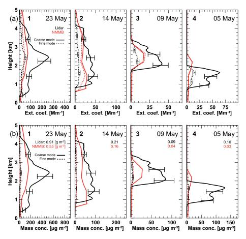
**Figure 7. (a)** Comparison fine (dotted) and coarse (solid) dust extinction coefficients derived from lidar observations (black) and simulated with NMMB/BSC-Dust (red). (b) Respective fine (dotted) and coarse (solid) dust mass concentrations derived from the lidar measurements (black) and simulated with NMMB/BSC-Dust (red). Column-integrated total dust mass concentrations are given as numbers.
