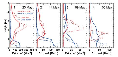
**Figure 5.** MACC/CAMS simulated marine (blue solid) and dust (red solid) contributions to particle extinction coefficient vs. respective lidar observations (dashed blue and red lines) for cases 1–4. Error bars show the overall retrieval uncertainty in the lidar observations. The variability in the modeled dust profiles around R/V *Meteor* are estimated to be 20–30 % (case 1), 10–20 % (case 2), 50–80 % (case 3), and 20–30 % (case 4; see text for more details).
