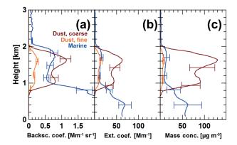
**Figure 4.** Solutions of the two-step POLIPHON data analysis (for case 4): (a) non-dust (blue, here for marine aerosol with lidar ratio of 20 sr), fine-mode dust (orange), and coarse-mode dust (dark red) backscatter coefficients, (b) respective marine, fine-mode, and coarse-mode dust extinction coefficients, and (c) marine, fine-mode, and coarse-mode dust particle mass concentration. Error bars indicate the retrieval uncertainties (1 standard deviation).
