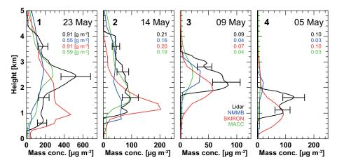
**Figure 6.** Dust mass concentration profiles observed with lidar (black, with retrieval uncertainty bars) and simulated with NMMB/BSC-Dust (blue), SKIRON (red), and MACC/CAMS (green) for cases 1–4. Column-integrated dust mass concentrations are given as numbers.
