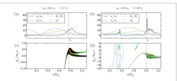
**Figure 7.** RSIT regime simulation ( $n_0 = 2.6n_c$ ,  $a_0 = 10$ ,  $\tau_r = 4$ , hydrogen): electron and ion density, electric field and vector potential amplitude for (a)  $t = 5\tau_L$  and (b)  $t = 15\tau_L$ . Electron distribution function  $f(x, p_x, t)$  and, when applicable, iso-contours of H' (black, solid lines), including the separatrices (red, dashed lines) in the lab frame for (c)  $t = 5\tau_L$  and (d)  $t = 16\tau_L$ .
