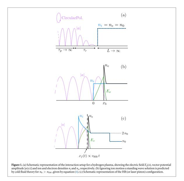
basis of the effect known as relativistic self-induced transparency (RSIT), in which a relativistically intense laser pulse ( $a_0 \gtrsim 1$ ) can propagate in a nominally overdense plasma.
