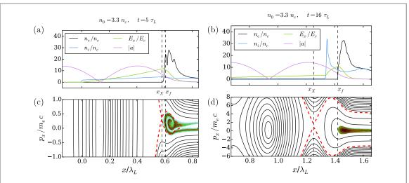
**Figure 6.** HB regime simulation ( $n_0 = 3.3n_c$ ,  $a_0 = 10$ ,  $\tau_r = 4$ , hydrogen): electron and ion density, electric field and vector potential amplitude for (a)  $t = 5\tau_L$  and (b)  $t = 15\tau_L$ . Electron distribution fuction  $f(x, p_x, t)$  and iso-contours of H' (black, solid lines), including the separatrices (red, dashed lines) in the lab frame for (c)  $t = 5\tau_L$  and (d)  $t = 16\tau_L$ .
