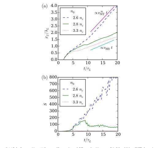
**Figure 3.** (a) Pulse front position  $x_f(t)$  for  $a_0 = 10$ ,  $\tau_r = 4\tau_L$  and different densities,  $n_0 = 2.6$ , 2.8 and 3.3  $n_c$  (RSIT, dynamic transition and HB regime, respectively). The upper and lower straight solid lines correspond to front propagation with  $v_{\text{SIT}}^{\text{ST}}$  (with  $n_0 = 2.6 n_c$ ) and  $v_{\text{HB}}$  (with  $n_0 = 3.3n_c$ ), respectively. (b) Cross-correlation function S(t) for the simulations of panel (a).
