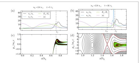
**Figure 8.** Dynamic transition regime simulation ( $n_0 = 2.8n_c$ ,  $a_0 = 10$ ,  $\tau_r = 4$ , hydrogen): electron and ion density, electric field and vector potential amplitude for (a)  $t = 5\tau_L$  and (b)  $t = 15\tau_L$ . Electron distribution fuction  $f(x, p_x, t)$  and iso-contours of H' (black, solid lines), including the separatrices (red, dashed lines) in the lab frame for (c)  $t = 5\tau_L$  and (d)  $t = 16\tau_L$ .
