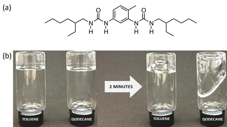
**Figure 1.** Structure of EHUT (a) and photographs of EHUT solutions in toluene or n-dodecane (b) 10 seconds (left) and 2 minutes (right) after inverting the vials ( $20\text{mmol L}^{-1}$ ,  $20\text{ }^{\circ}\text{C}$ ).
