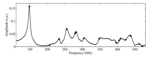
Figure 3. A typical resonant spectrum measured on a bone specimen. The plus signs (+) represent the extracted resonant frequencies.
