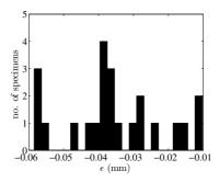
Figure 7. The distribution of the dimension error  $\epsilon$  obtained by comparing for each specimen the volume of the bone SR- $\mu$ CT reconstruction and the volume of a hypothetical RP of dimensions  $\dim^{exp} \pm \epsilon$ .
