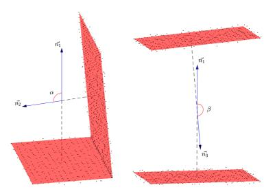
Figure 5. The angle  $\alpha$  is defined by the angle between the normal  $(\vec{n_1} \text{ and } \vec{n_2})$  of two adjacent faces which are found by fitting the cloud of points (the dots in the figures) with the equation of the best plane in the least-square sense; accordingly,  $\beta$  is defined by the angle between the normal  $(\vec{n_1} \text{ and } \vec{n_3})$  of two opposite faces. For a perfect RP,  $\alpha$  and  $\beta$  should equal to 90° and 180°, respectively.
