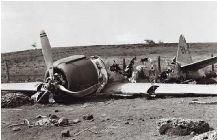
Fig. 7.1 The burned Zero fighter aircraft on the island of Niihau. The 20mm cannon of the left wing have been removed.
