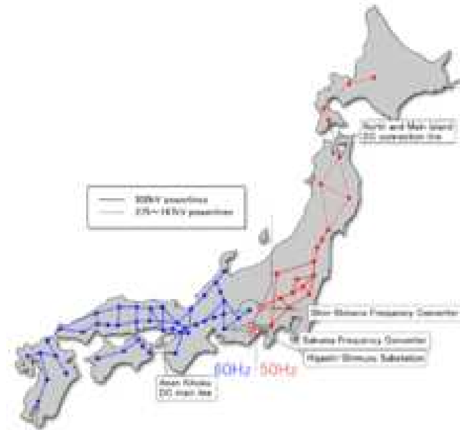
Fig. 6.x Electric network of Japan. The Japanese electric network is divided into two parts: the 50 Hz north-east part and the 60 Hz south-west part. This is a fairly rare case among developed countries. Source: Wikipedia article entitled "Fukushima Daiichi nuclear disaster")
