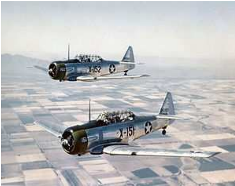
Fig. 2.4c AT-6 light attack aircraft. The AT-6 has up to 3 (7.62 mm=0.30 inch) machine guns; its range is 1,175 km. Its first flight was in 1935 and it is still in use in 2012; some 15,500 have been built. Source: Wikipedia, article entitled “North American T-6 Texan”.
