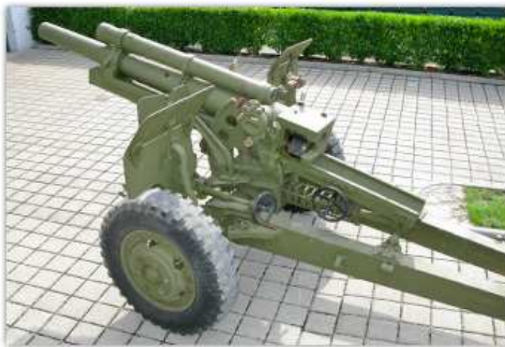
Fig. 6.7 105-mm howitzer. A howitzer is a gun which fires shells at fairly steep angles. It is intermediate between a gun which has high velocity and relatively flat trajectories and a mortar which fires at very steep angles. In almost horizontal position the 105-mm can be used for direct hits with a range of about 1 km. In a steep position, i.e. when really used as a howitzer, the range is about 3 km. Between July and October 1948 a few battalions of the Korean Constabulary received training in the use of machine guns, 57-mm anti-tank guns and 105-mm howitzers. Source: http://www.asphm.com
