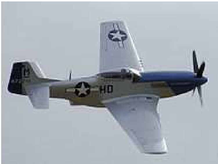
Fig. 2.4b P-51 Fighter aircraft. The P-51 had 6 Browning machine guns mounted in the wings which could fire about 7 rounds per second. It had a range of 1,865 km with external tanks. Source: Wikipedia, article entitled “North American P-51 Mustang”.
