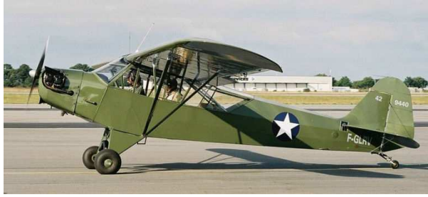
Fig. 6.13 Piper L-4 Grasshopper. The Piper L-1 to L-5 were military versions of the Piper Cub. The designation “L” means Liaison aircraft.
