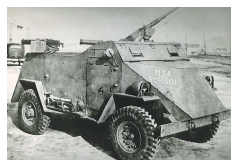
Fig. 2.3 Scout car S1. There is a Browning M2 machine gun on top and two Browning M1921 machine guns in rear. Source: http://ww2db.com/image.php?image_id=7960
