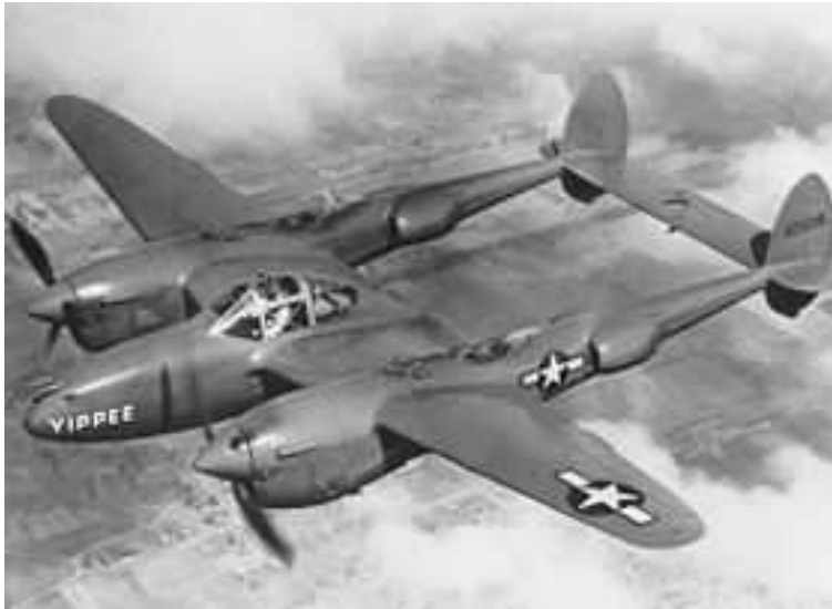
Fig. 2.4a P-38 Fighter aircraft. The P-38 had 4 Browning machine guns mounted in the nose which could fire about 7 rounds per second. It had a range of about 2,000 km. Source: Wikipedia, article entitled “Lockheed P-38 Lightning”.
