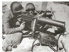
Fig. 2.2 Water cooled machine gun. The picture shows a 0.30 inch water-cooled machine gun which was used in World War II. There was also a similar air-cooled 0.30 machine gun. Source: http://www.rt66.com/korteng/SmallArms/30calhv.htm
