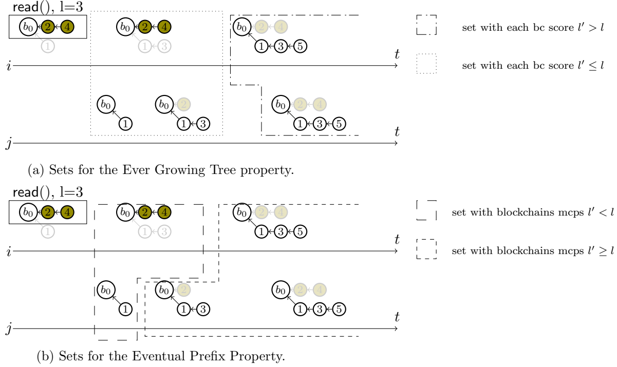
Figure 3: Concurrent history that satisfies the Eventual BT consistency criterion. In such scenario f selects the longest blockchain and the blockchain score is the length l . In case (a) and case (b) the concurrent history is the same but different sets are outlined.
