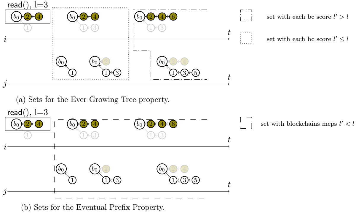
Figure 4: Concurrent history that does not satisfy any BT consistency criteria. In such scenario f selects the longest blockchain and the blockchain score is the length l .
