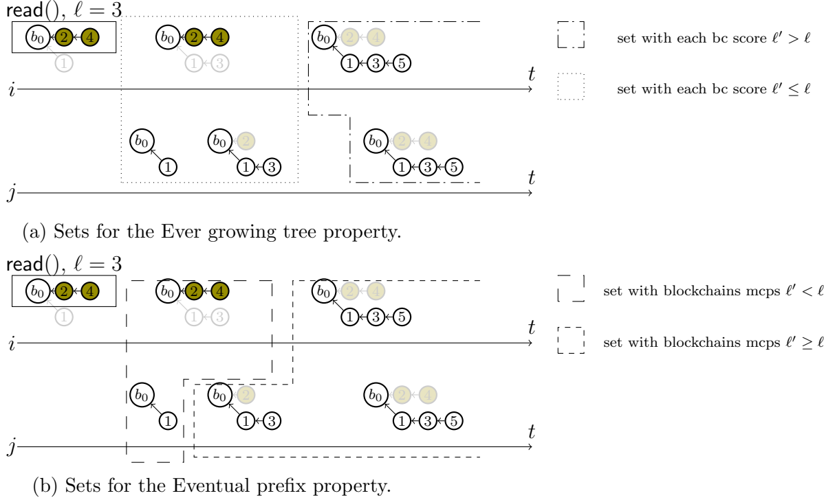
Figure 3: A concurrent history that satisfies the Eventual BT consistency criterion. In this scenario function f selects the longest blockchain and the blockchain score is the length \ell . In both cases (case (a) and case (b)) the concurrent history is the same but different sets are outlined.
