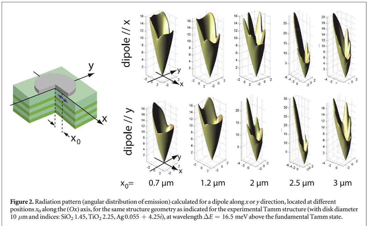
**Figure 2.** Radiation pattern (angular distribution of emission) calculated for a dipole along  $x$  or  $y$  direction, located at different positions  $x_0$  along the  $(Ox)$  axis, for the same structure geometry as indicated for the experimental Tamm structure (with disk diameter  $10 \mu\text{m}$  and indices:  $\text{SiO}_2$  1.45,  $\text{TiO}_2$  2.25,  $\text{Ag}$  0.055 + 4.25*i*), at wavelength  $\Delta E = 16.5 \text{ meV}$  above the fundamental Tamm state.
